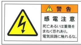
Indicates that improper use may cause an electric shock.
