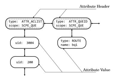
The attribute list data is dynamically made in the heap area, it is necessary to free by NQSafree0 function.
