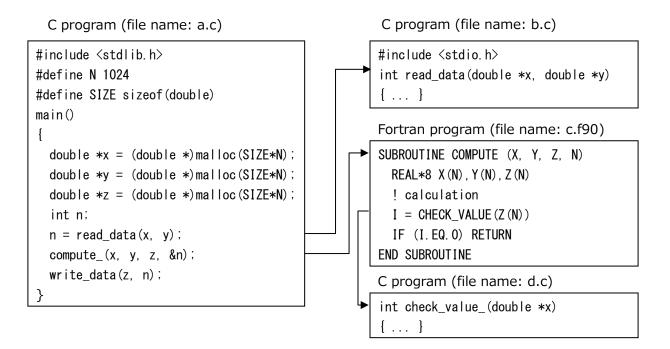
In this example, a Fortran program is called from a C program, and a C program is called from a Fortran program. When these programs are called, the function name and procedure name coded in the program are converted into an external symbol name, and the data is shared between C and Fortran by passing arguments or return values.
