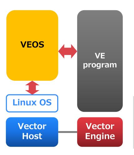
VEOS features: VE program loading System call handling VE process management VE memory management Signal handling OS commands supporting gdb, ps, free, top, sar etc.
