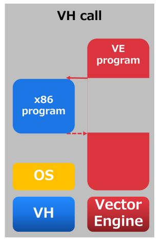
"VE offload" offloads compute kernels from x86 to VE
